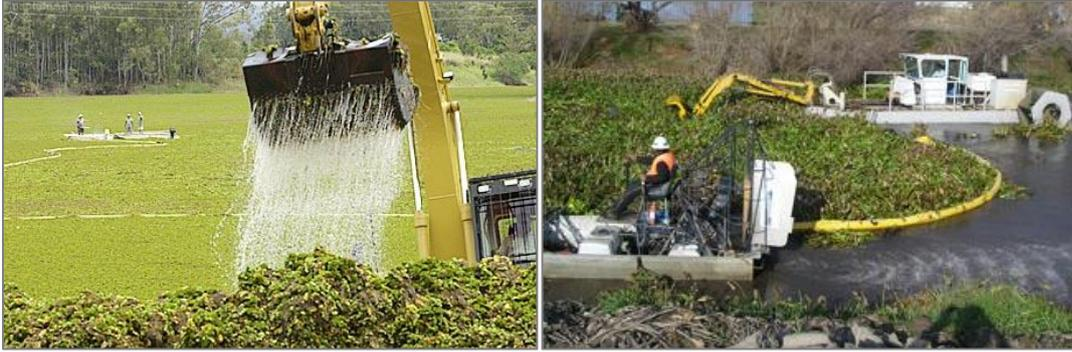
The photos above show two examples of large scale mechanical removal machinery which would be unsuitable for use at Te Henga.
